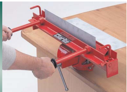
Chassis repairs mean that you need to fold steel - this is a Clarke bench folder - but you can make your own folder out of angle iron
